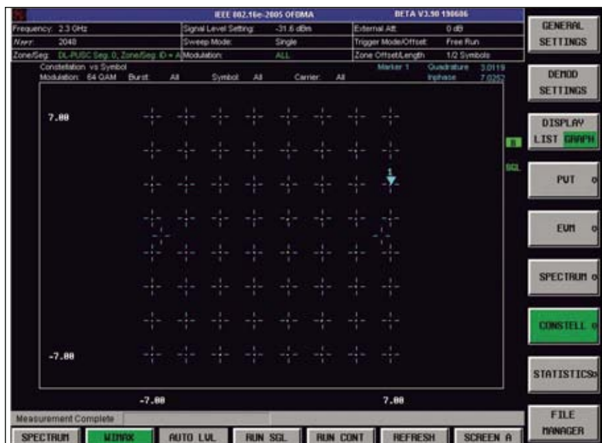
▲ Fig. 1 Constellation diagram of a 64QAM WiMAX signal demodulated by a signal analyzer.
